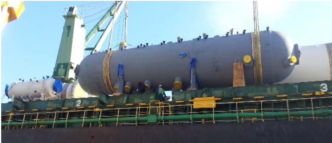
STEAM DRUM OF WHB - PARDIS 3RD UREA & AMMONIA, IRAN
