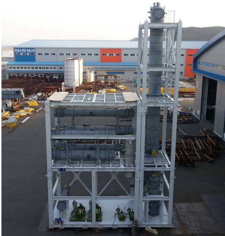
BENZEN STRIPPER PACKAGE - INTECSA SABIC SK WWT PROJECT IN SAUDI ARABIA
