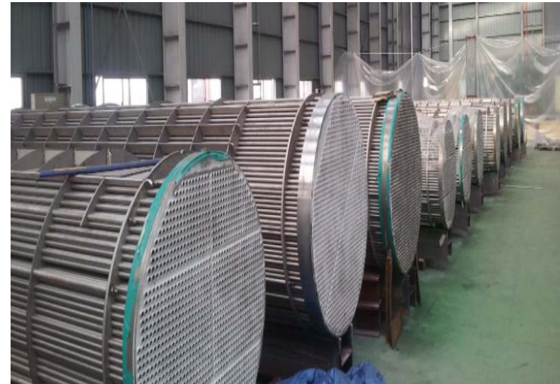
TUBE BUNDLES OF TITANIUM HEAT EXCHANGER - PGSOC / BANDAR ABBAS G&C PROJECT, IRAN
