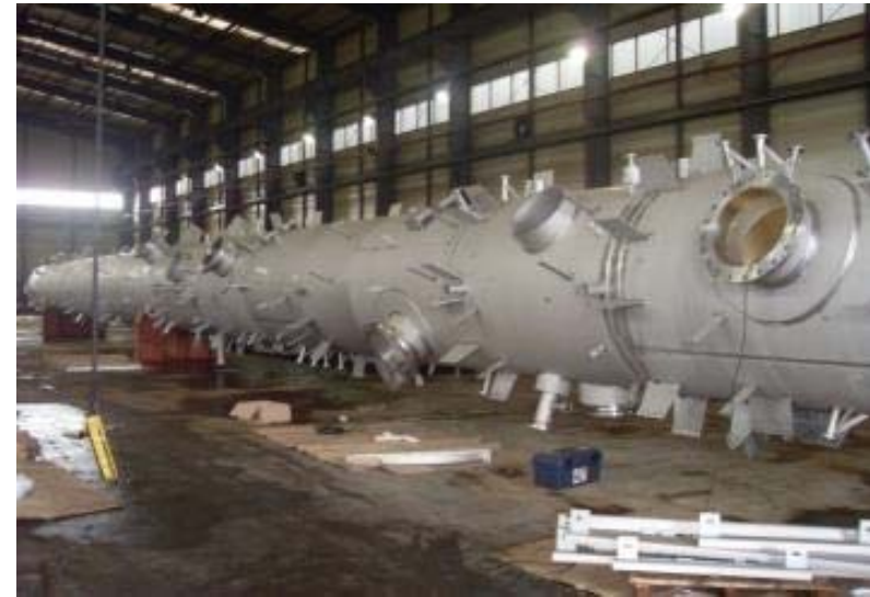
DEMETHANIZER - SECL MOC PROJECT IN THAILAND
