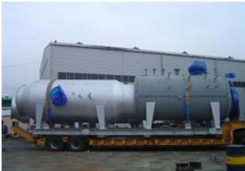
THERMAL REACTORS W/WHB - JGC/SOHAR REFINERY, OMAN
